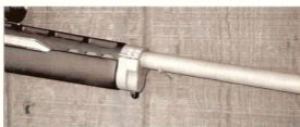
This is the Accuracy Systems gas block with sling swivel stud. Note the Douglas Premium Match Grade barrel and the matte gray finish, which is excellent for low visibility.
